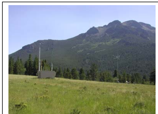
This Rocky Mountain National Park air quality monitoring station measures ozone, elements of visibility, other gaseous pollutants and meteorological events.
